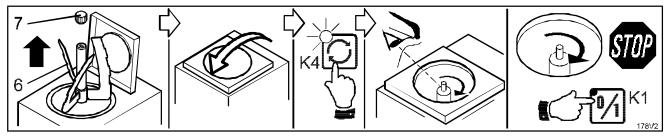
Open the lid, unscrew the fixing knob [7], pull out the beater [6] from the cylinder, then close the lid.
