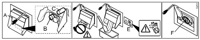
The extraction door chute has a tilting protection flap [A]. The product during extraction lifts this. The flap together with the fixed grill [F] prevents fingers or objects from being **ACCIDENTALLY** inserted through the extraction door.
