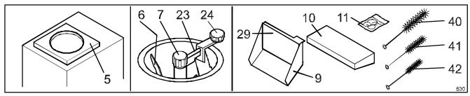
Check that the machine is supplied with the lid [5] and that the beater [6] is correctly fixed inside the cylinder with its knob [7]. The bigger models are supplied with a tilting blade [23] and its fixing knob [24].
