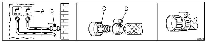
Use linen-rubber tubes for water connection, arranged for 15 Bar pressures, interposing a valve or a faucet [B] **ABOVE** the delivery pipe; use a 3/4" rubber holder [C], well fixed with a proper band [D] to connect the tubes at the device's union.
