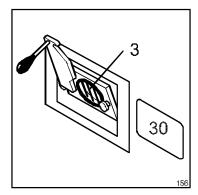
In some models, a fixed protection grill [3] prevents fingers or objects from being **ACCIDENTALLY** caught inside the extraction chute. In order to insure normal operation it is not possible to adjust the fixed grill as to prevent fingers and objects from being **VOLUNTARILY** inserted through the extraction chute (according to Machines Directive 89/392/CEE and ensuing modifications, Appendix I, Art. 1.1.2.b, 3<sup>rd</sup> paragraph).
